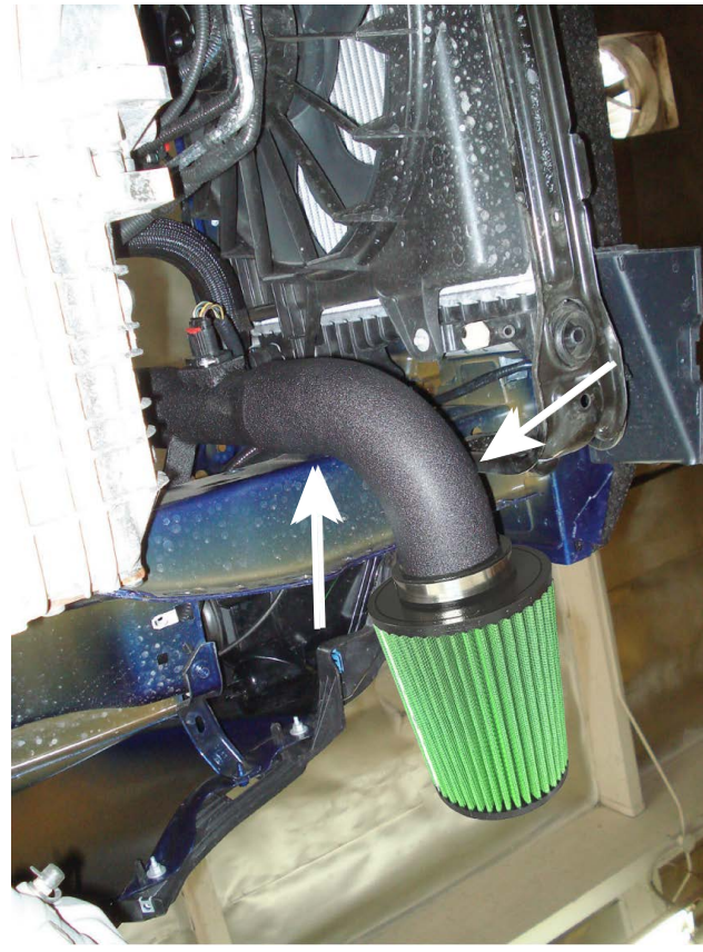
Figure 12. Adjust for proper clearance.
